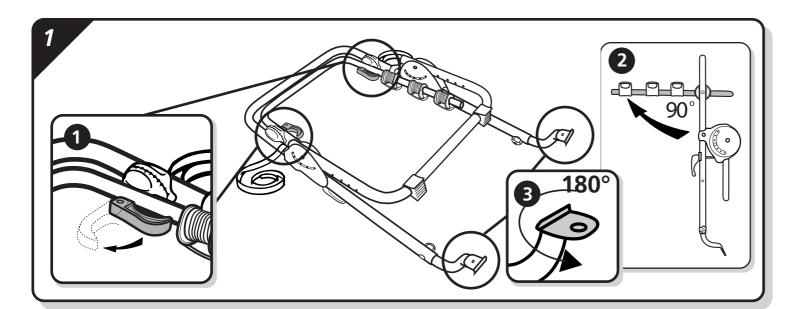
Position the assembled carrier on a clean surface as illustrated. (1) Release the 2 adjuster levers and (2) rotate the cycle support arms through 90° and lock in position. The quick release action should be
